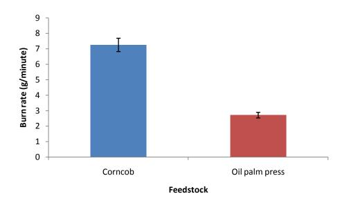
Figure 5. Mean burn rate of corn cob and oil palm press. Error bars represent S.E at P < 0.05.
