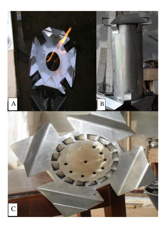
**Plate 1.** Features of the Lucia biomass stove: (A) stove in use; (B) side view of stove; and (C) stove bottom showing primary air inlet
