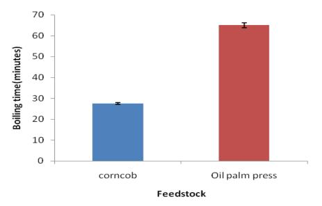
Figure 2. Influence of corn cob and oil palm press on boiling duration of water. Error bars represent S.E at P < 0.05.
