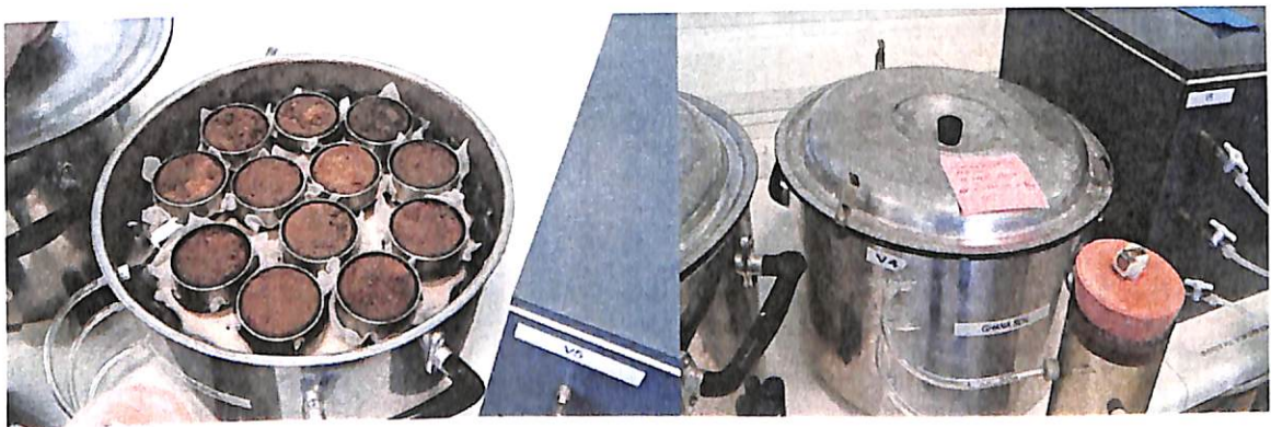
Figure 8: Suction plates for regulation of matric potential at pF 2.5 and 2.7.
