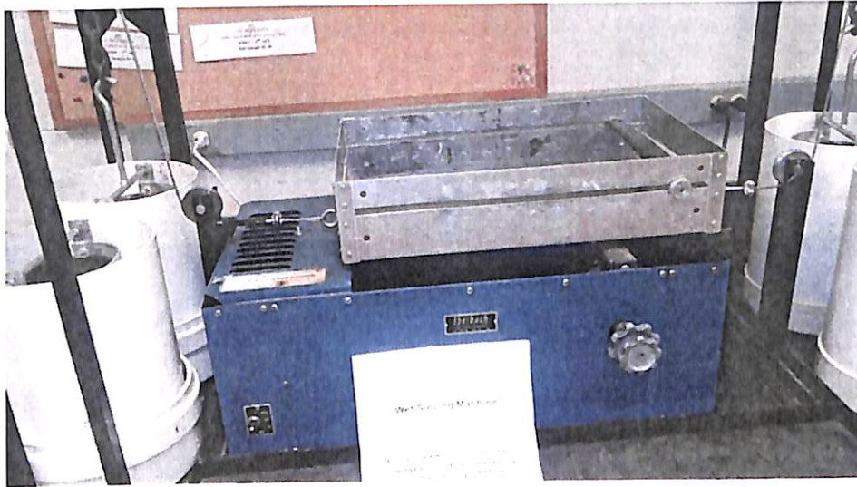
Figure 4: The wet sieving machine.
