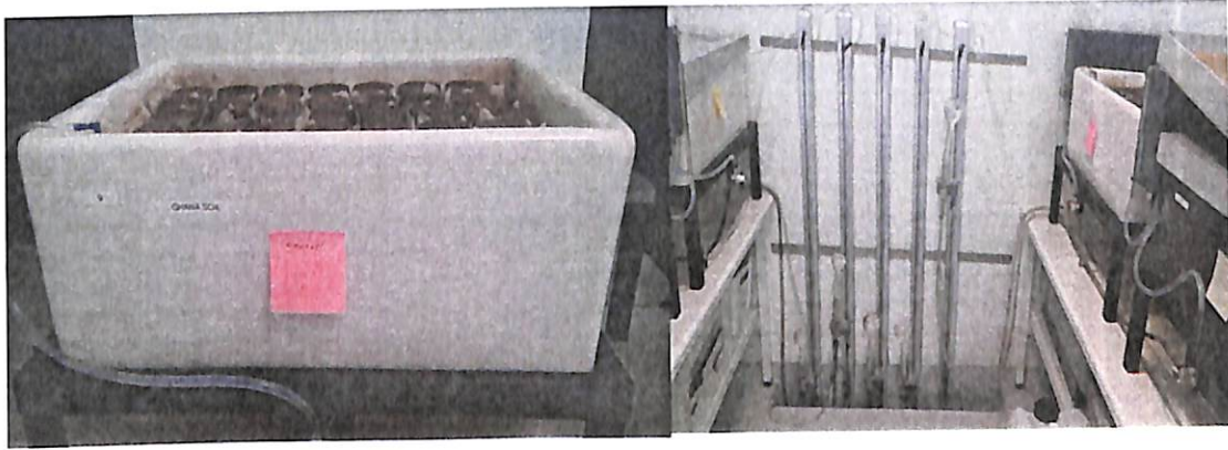
Figure 7: Sand box for the regulation of matric potential between pF 1 and 2.0.
