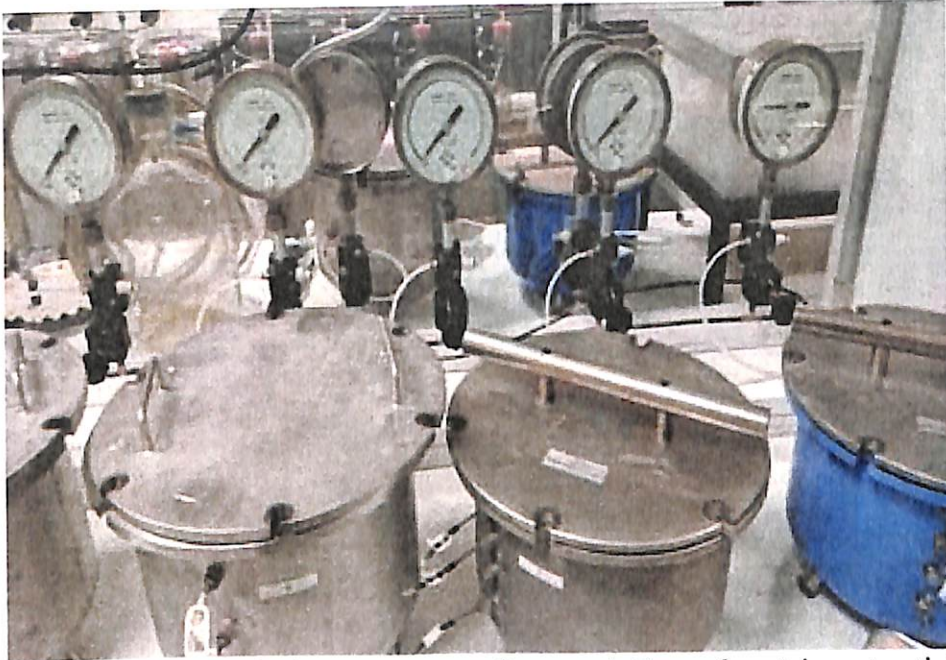
Figure 9: Richard plate apparatus for regulation of matric potential at pF3.0.
