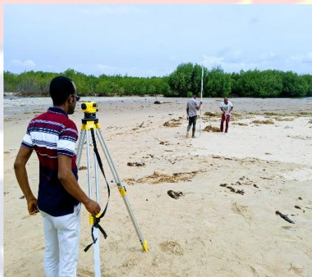
Beach Profile using a Dumpy Level
