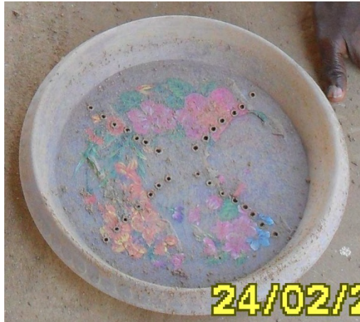
Plate 4a: Plastic bowl used for Germination test (5 cm deep and 30 cm wide)
