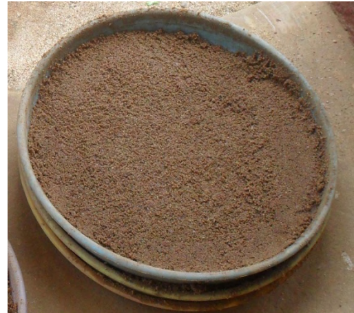
Plate 4b: Plastic bowl filled with sand to a depth of 3.5 cm leaving 1.5 cm space above.
