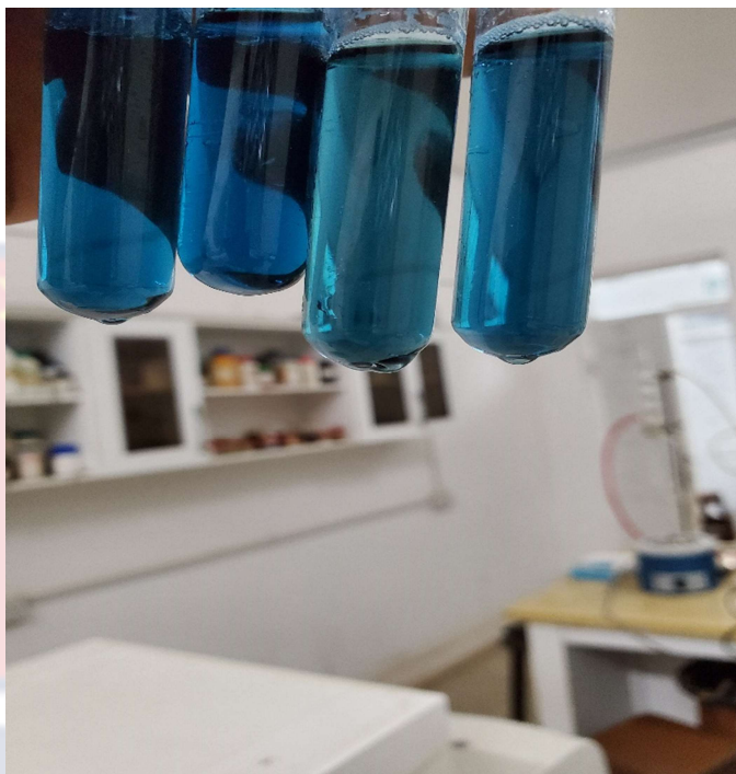
Figure 12: Colour formed from reaction of sample protein with Bradford reagent.
