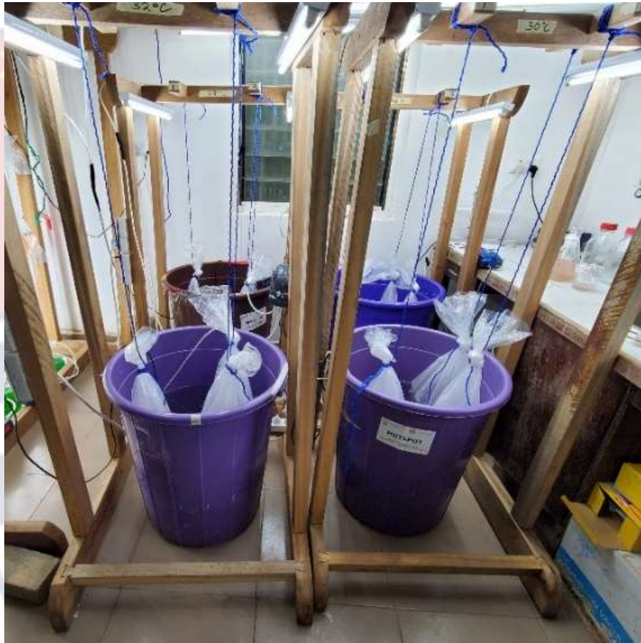
Figure 10: Experimental setup showing suspended culture bags, water bath and light supply.
