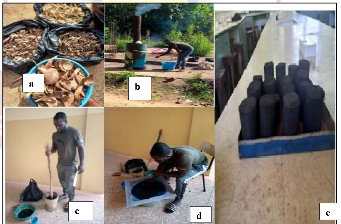
Figure 7: Composite biomass preparation stages, (a) dried feedstocks before pyrolysis (b) pyrolysis (c) particle size reduction (d) Screening and (e) Composite biomass briquettes
