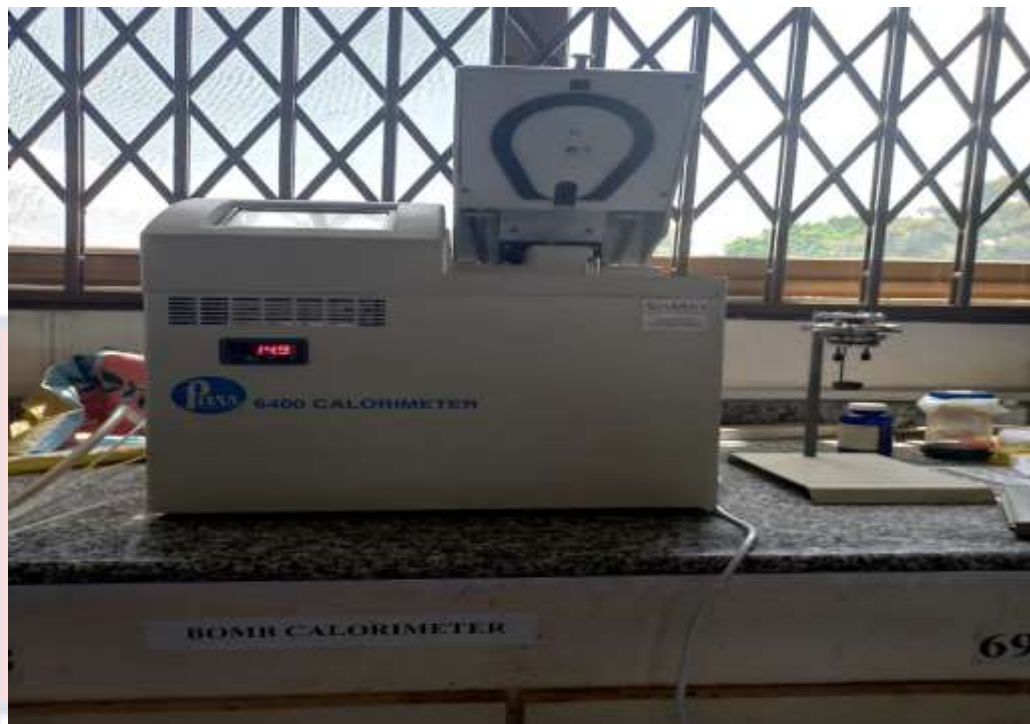
Figure 9: Parr 6400 Bomb Calorimeter used to estimate the gross calorific value of composite biomass briquette.
