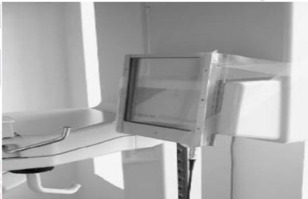
Figure 9: Set-Up for DAP Measurement (Image is from Field Work)
