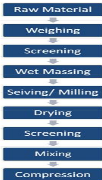
Figure 3: Flowchart for processing Steps in Wet Granulation powdered sachets
