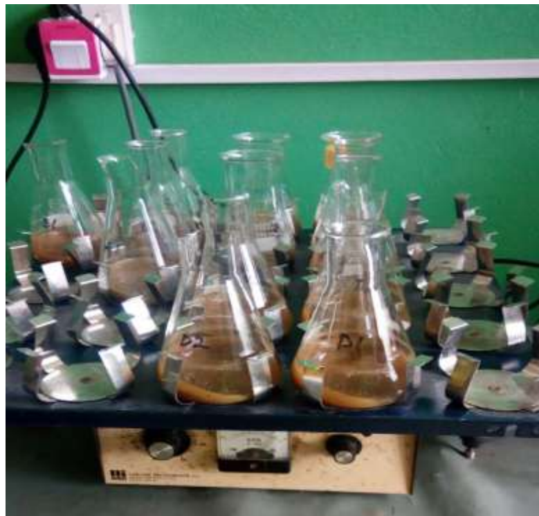
Plate 9: Pre-digestion of smoked fish powder on gyration shaker.
