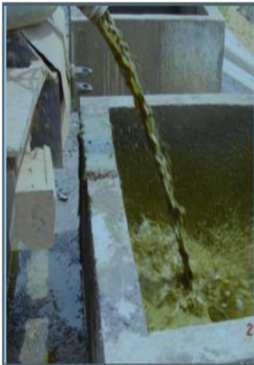
Fresh FS collected from unsewered public toilets unloaded at Buobai FS treatment plant, Ghana. (Source: Eawag/Sandec, 2003)
