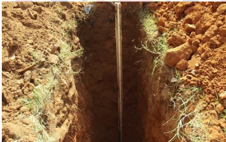
Plate 6. 5: Soil profile tests pits at LLSite1
