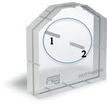
Figure 17: Wilke phantom with defined length dimension
