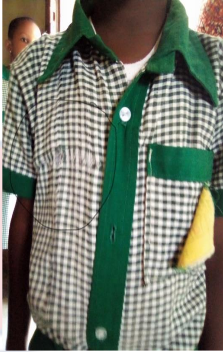
PKG 1 yarns slipped at front
