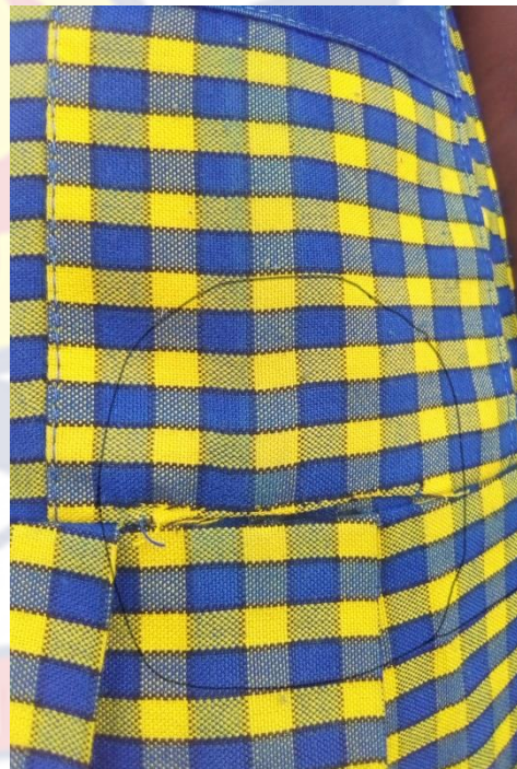
PKG 2 yarns slipped at pocket
