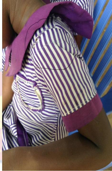
PKG 6 yarns slipped at shoulder
