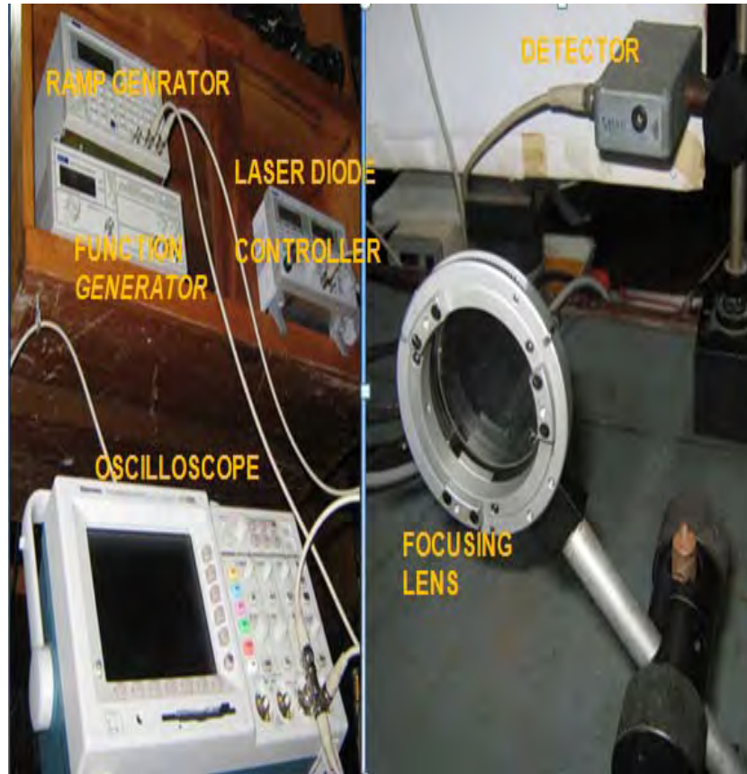
Plate 2: Some of the equipment used for the wavelength modulation spectroscopy set-up.
