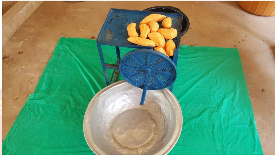
Locally design chipping machine – cut sweet potatoes into chips
