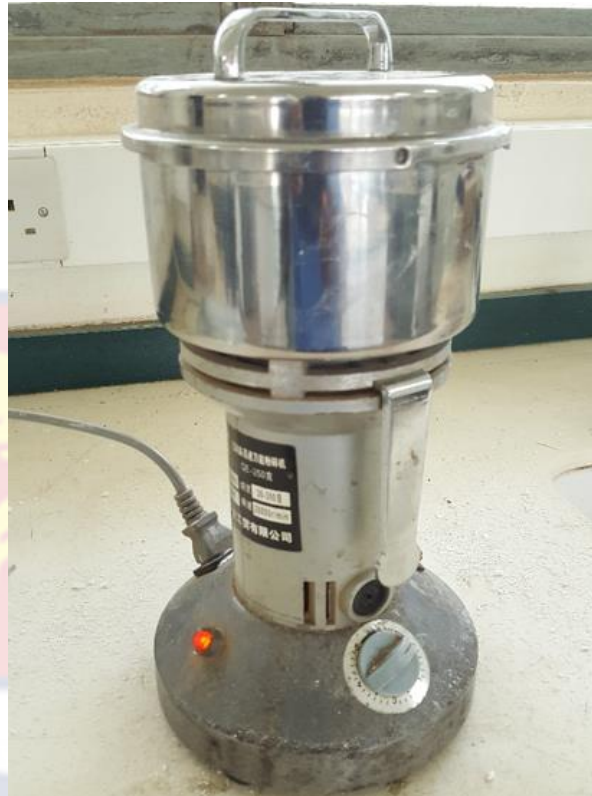
Power grinder – for milling dried cassava pulp
