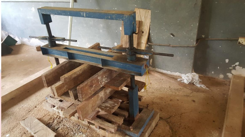
Double screw press – for removing water from the milled cassava pulp
