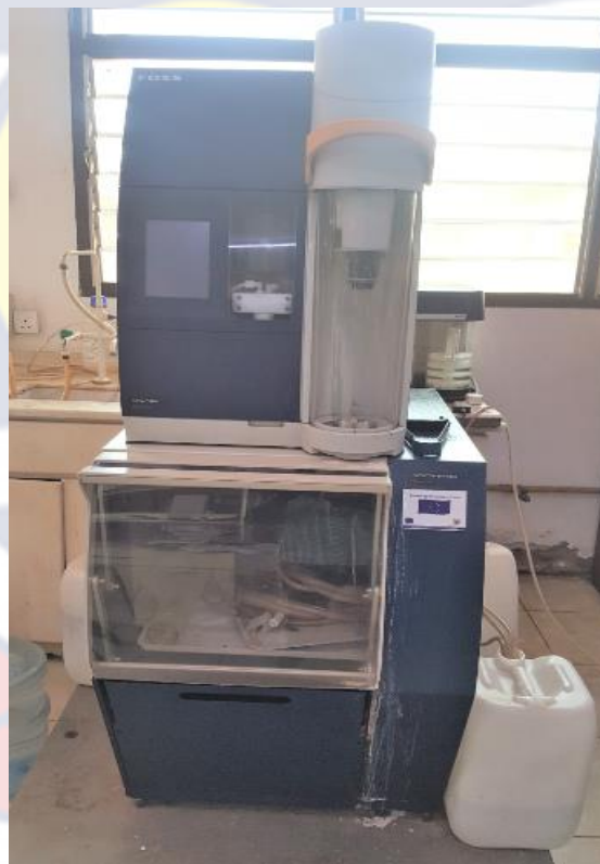
Tecator Kjeldtec systems (Kjeltec 8400) – for protein content determination
