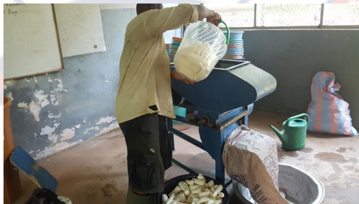
Feeding the hopper of the cassava grater with cassava sample for milling
