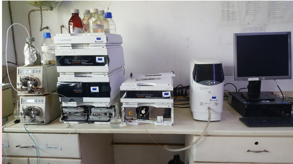
HPLC equipment – for analyzing aflatoxin in cassava flour and OFSP flour samples
