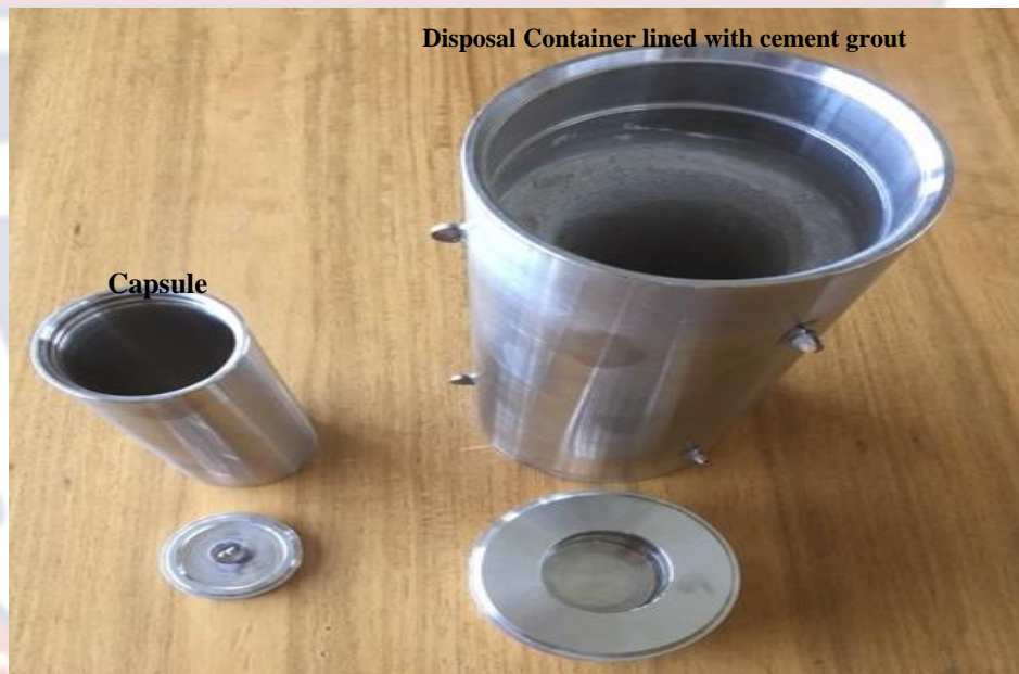
Figure 12: Stainless steel capsule and disposal container lined with cement grout (containment barrier) (IAEA, 2017).
