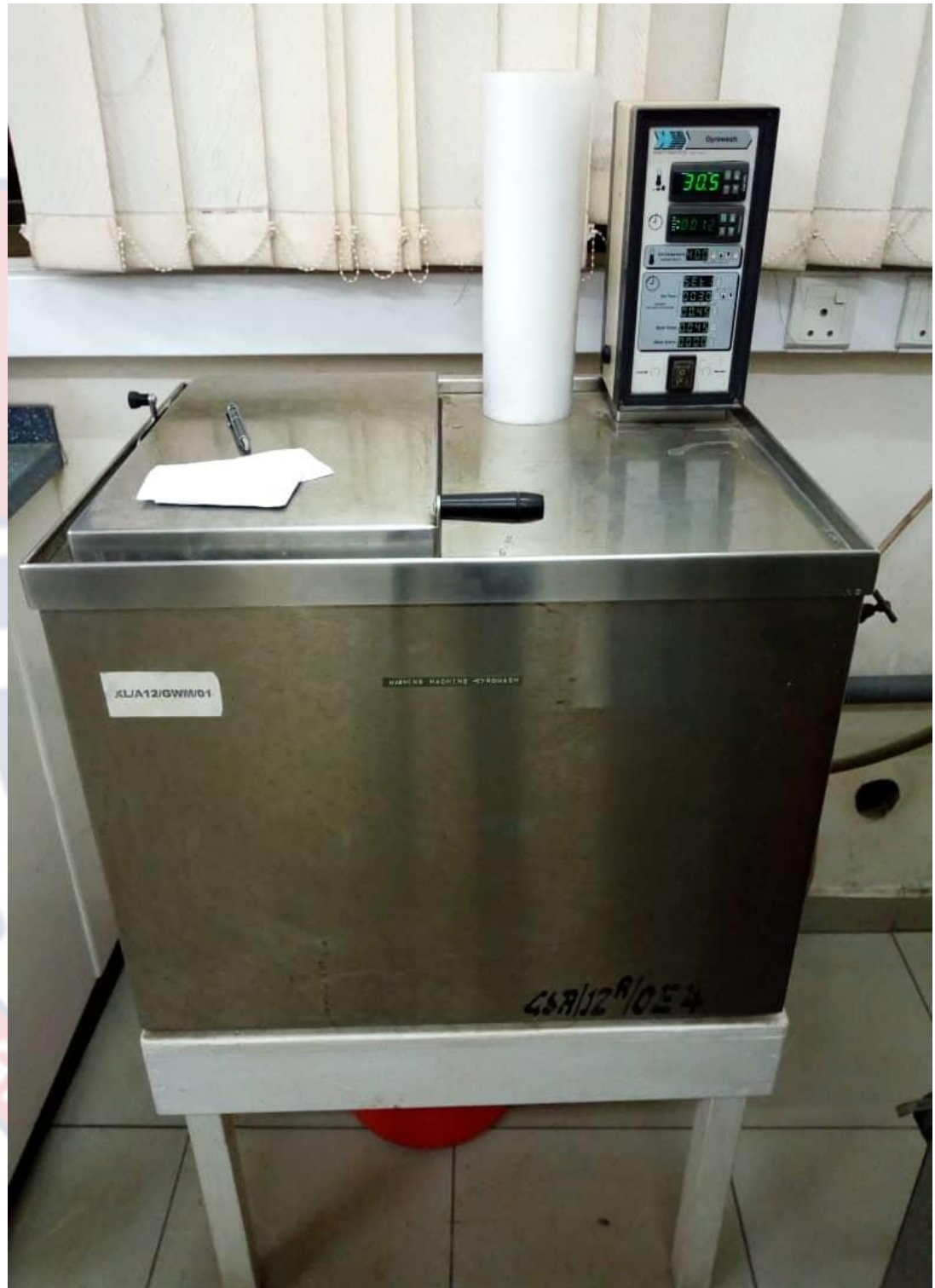
A Standard Laundry-Ometer (Gyrowash SN: 315/8/98/5040)
