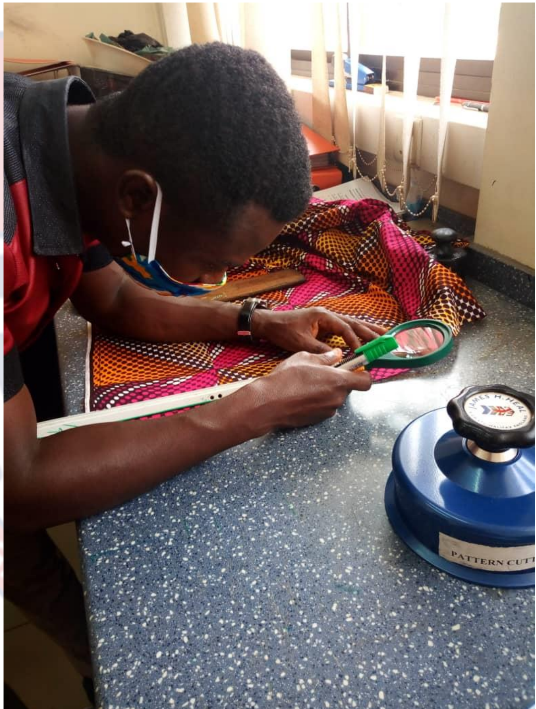
Identifying weave type with the hand magnifying glass (eye piece)
