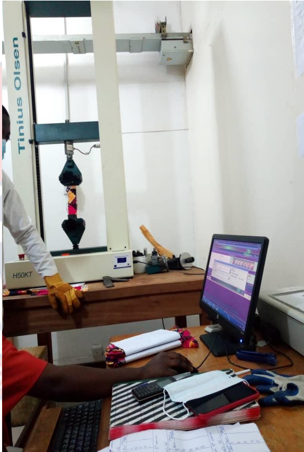
Testing of tensile strength of specimens with Hounsfield H50KT
