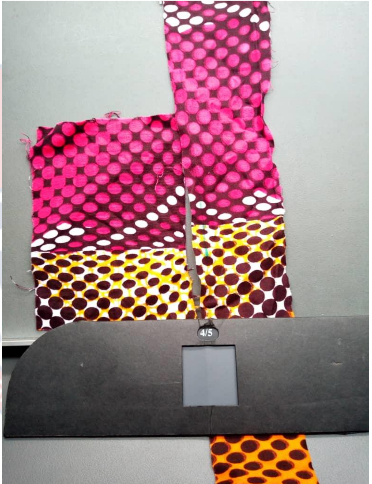
Assessing the colour of specimens with the assessment colour chamber and a geometric grey scale
