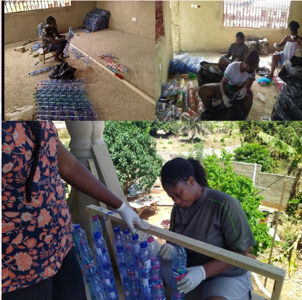
Figure 4.0.21. Images at the top left and right depict the preparation of the 'silk' for later spinning of the 'web' – the stringing process. The bottom image shows the spinning of the web by passing the cords through the drilled holes in the frames to be fastened by tying two separate cords through the drilled holes in the frames to be fastened by tying two separate cords into a knot. Source: Mawukplorm H. Adjahoe (2021)
