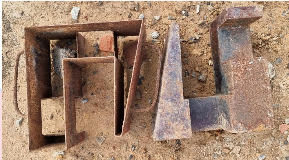
Figure 4.0.9. This image reveals a hollow mould and a solid mould. As a part of the experimentation process, the bottom of one of the moulds was removed to extricate the molten-plastic-sand cast. Source: Mawukplorm H. Adjahoe, waste designing (2021)
