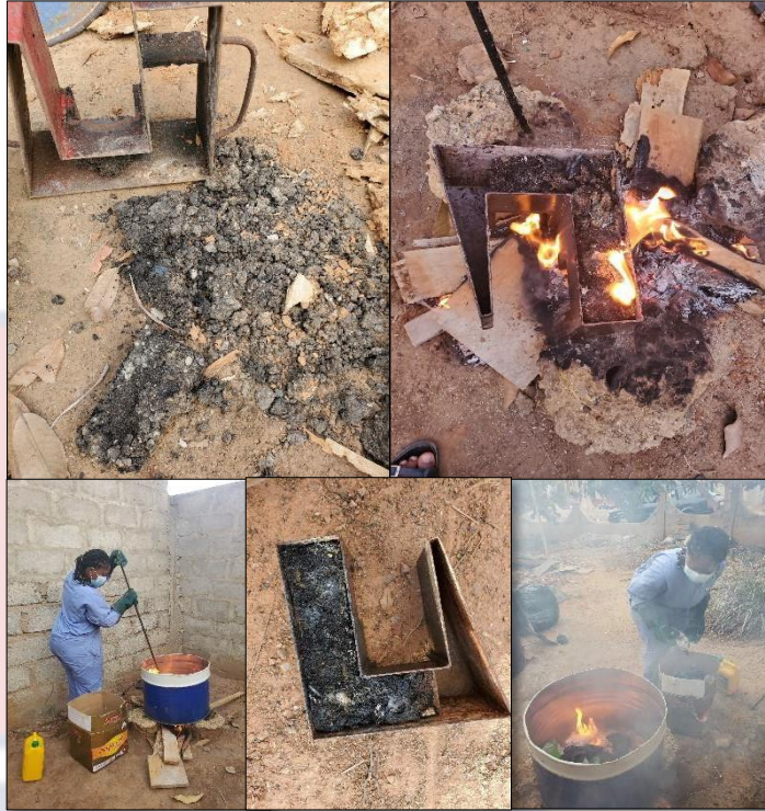
Figure 4.0.11. The process of creating the molten-plastic-sand block. This method was unfeasible considering the health hazards it posed coupled with the amount of time required to cast one block. Source: Mawukplorm H. Adjahoe, waste designing (2021)
