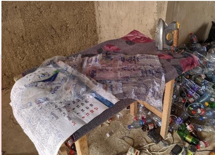
Figure 4.0.19. Process of building the plastic sheet through the act of ironing series of plastic sachet which have been cut open and aired to produce a dry surface. Source: Mawukplorm H. Adjahoe (2021)
