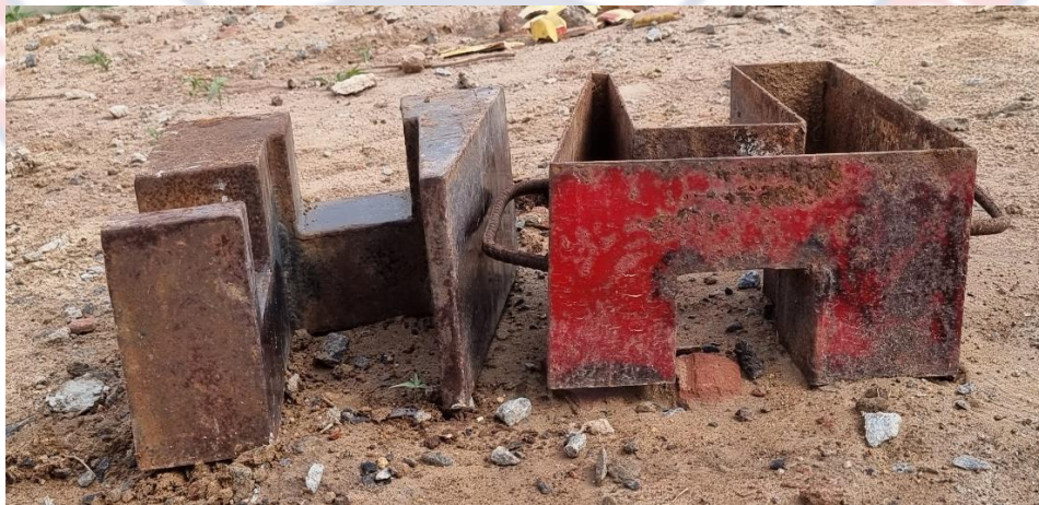
Figure 4.0.8. Picture of moulds after they have gone through some levels of heat. Source: Mawukplorm H. Adjahoe, waste designing (2021)
