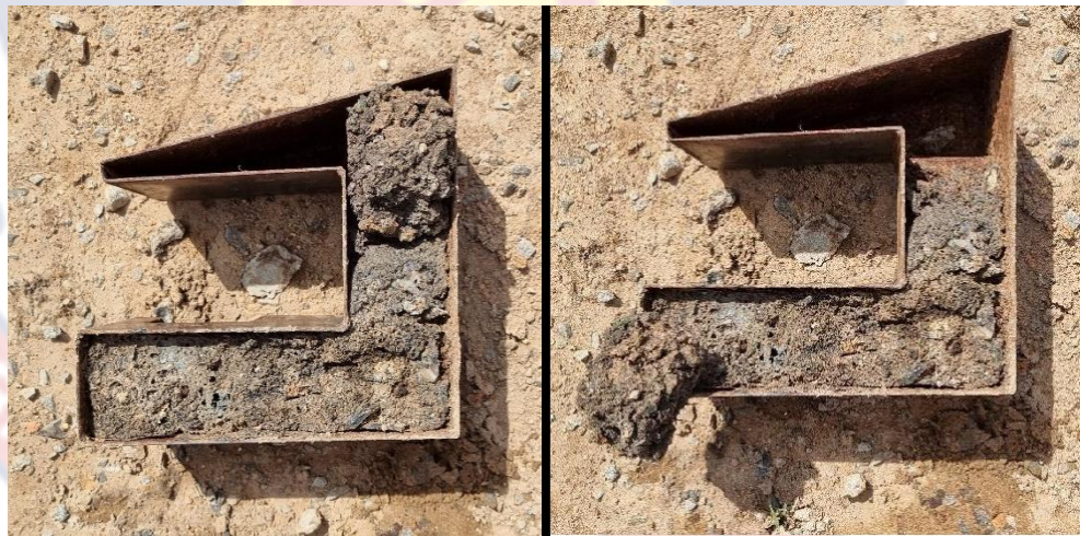
Figure 4.0.12. The result of experimenting with melting plastics mixed with sand to cast a block, which resulted in the removal of the bottom of the mould to be able to remove the block. Source: Mawukplorm H. Adjahoe (2021)
