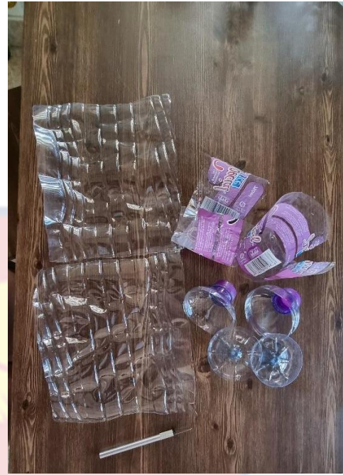
Figure 4.0.17. The layout of the flattened bottles together with their removed parts. The body cylinders are flattened out but are not in themselves flat, and were light in weight. Source: Mawukplorm H. Adjahoe (2021)
