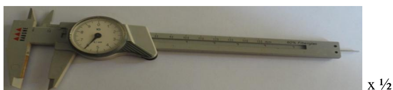
Plate 4: A pair of Vernier calipers used to measure the diameters of the clear zones
