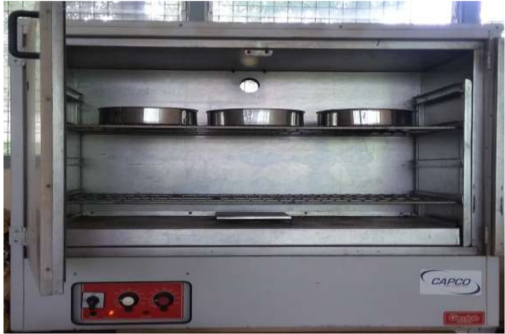
Figure 2: Arrangement of sample holders in the cabinet hot air dryer Microwave Alone Drying
