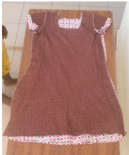
VIII. Associated constructional problems of design 1 (uneven side seam allowance and hem)
