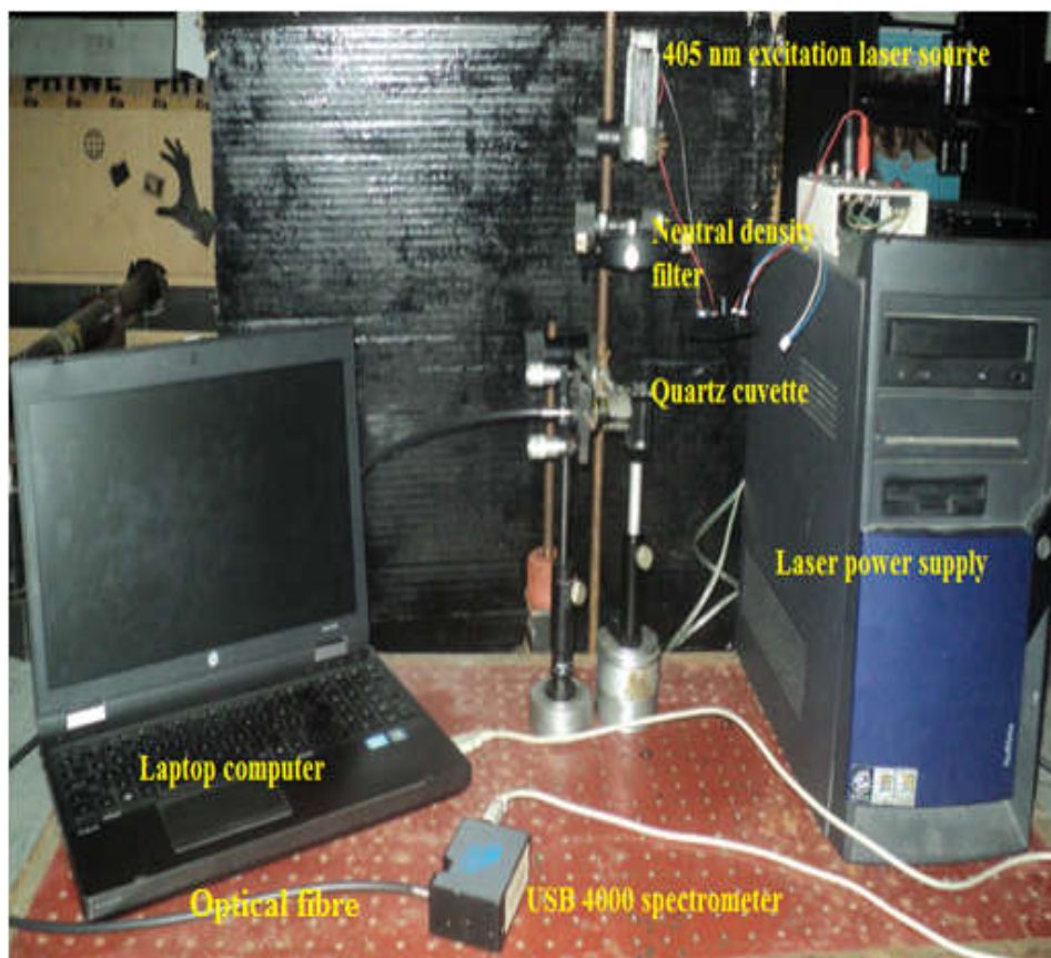
Plate 2: A photograph showing the components of the set-up for acquiring fluorescence spectra data.
