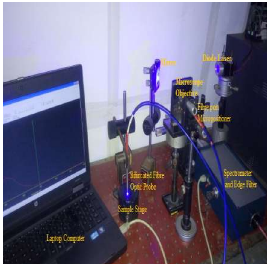
Plate 6: Photograph Showing the Components of the Laser – Induced Autofluorescence (LIAF) Set-Up for Acquiring Autofluorescence (AFS) Spectra Data.
