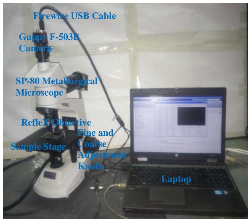
Plate 4: Photograph of the Multispectral Light Emitting Diode (LED) Imaging (MSLEDI) Microscope (MSLEDIM Set-Up) at the Laser and Fibre Optics Centre (LAFOC), Department of Physics, School of Physical Sciences, College of Agriculture and Natural Sciences, University of Cape Coast, Cape Coast.
