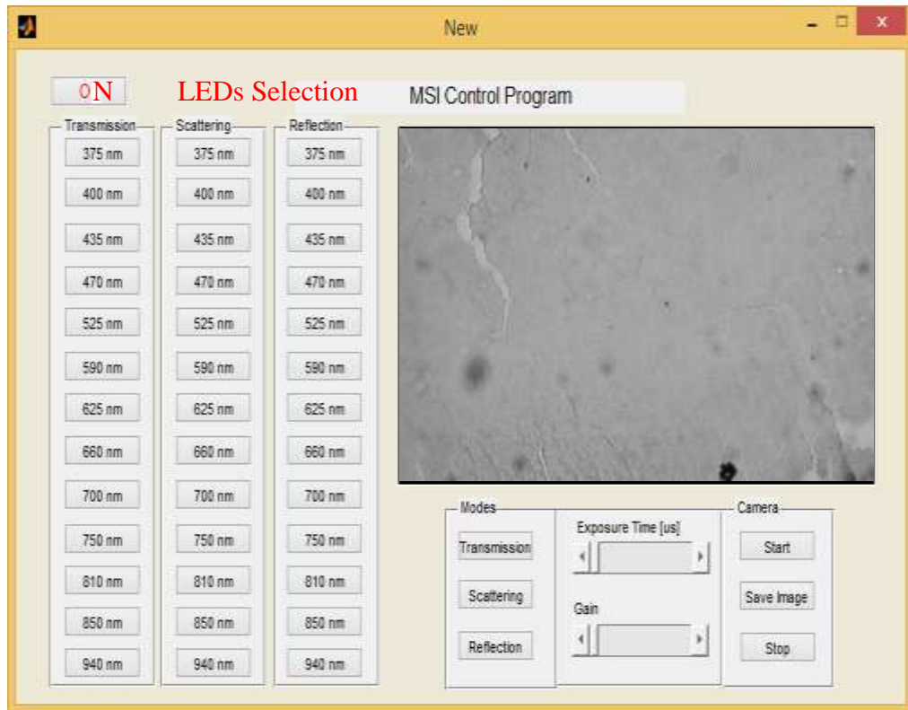
Plate 5: Graphical User Interface (GUI) of Matlab Program for Controlling the Light Emitting Diodes (LEDs) and Capturing Images from the Imager with an Image from the 590 nm LED.
