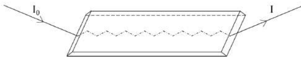
Figure 4. Schematic Figure Illustrating the ATR Technique where the Infrared Beam is Totally Reflected Several Times Inside the ATR Crystal. I_0 and I are the Intensity of the Infrared Beam Before and After the Interaction with the Sample Respectively.
