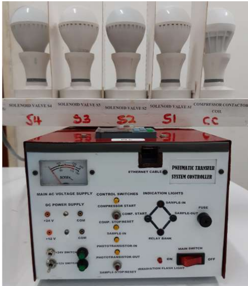
Figure 65: PTS controller with bulbs to simulate the solenoid valves.
