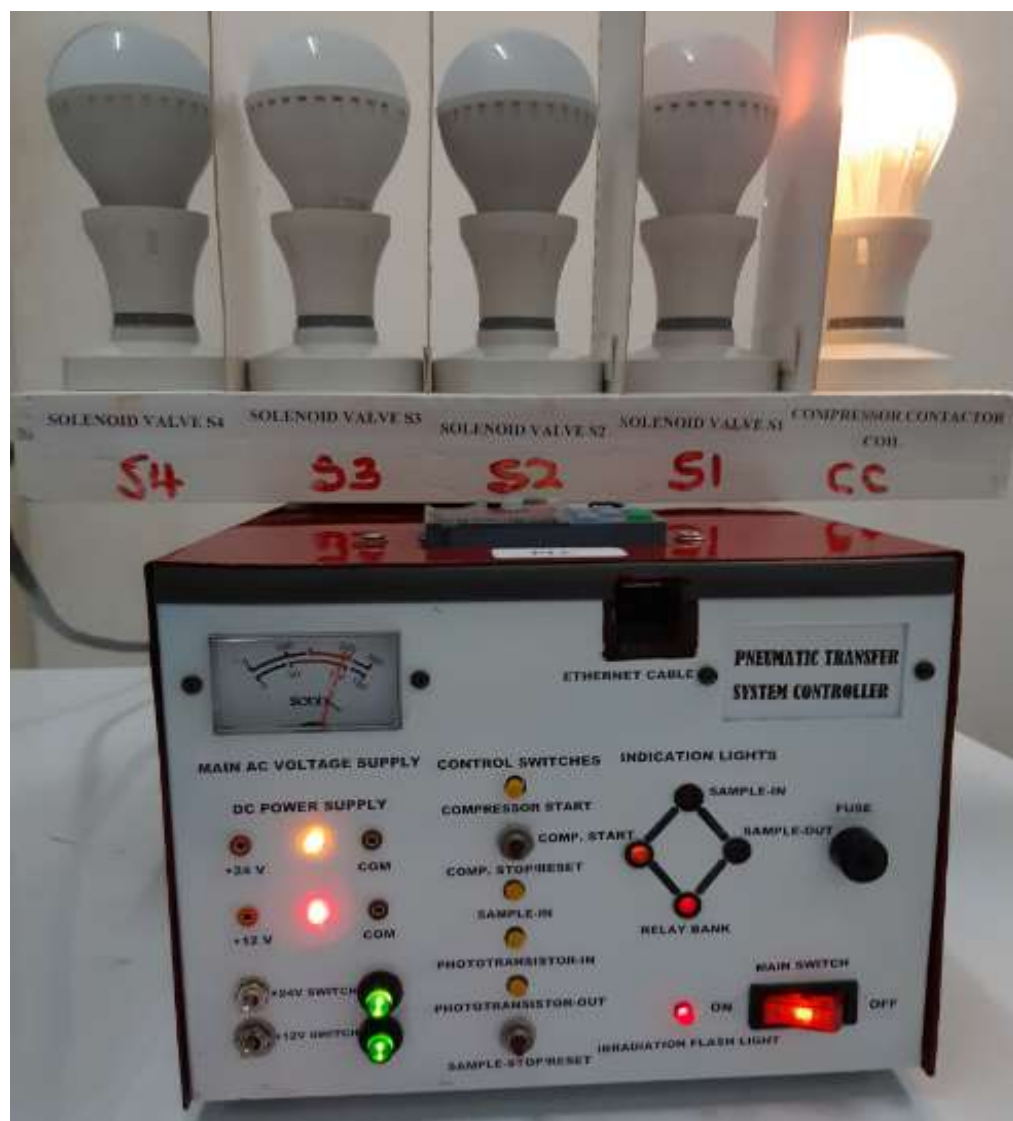
Figure 75: Solenoid valves S 1 and S 3 close; sample irradiation starts with flash light / beeps of buzzer.
