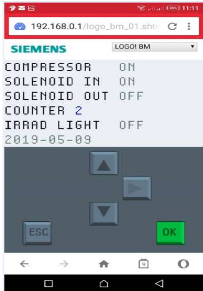
Figure 87: Irradiation cycle repeated, counter recorded the two samples for the cycles (monitored from mobile phone).
