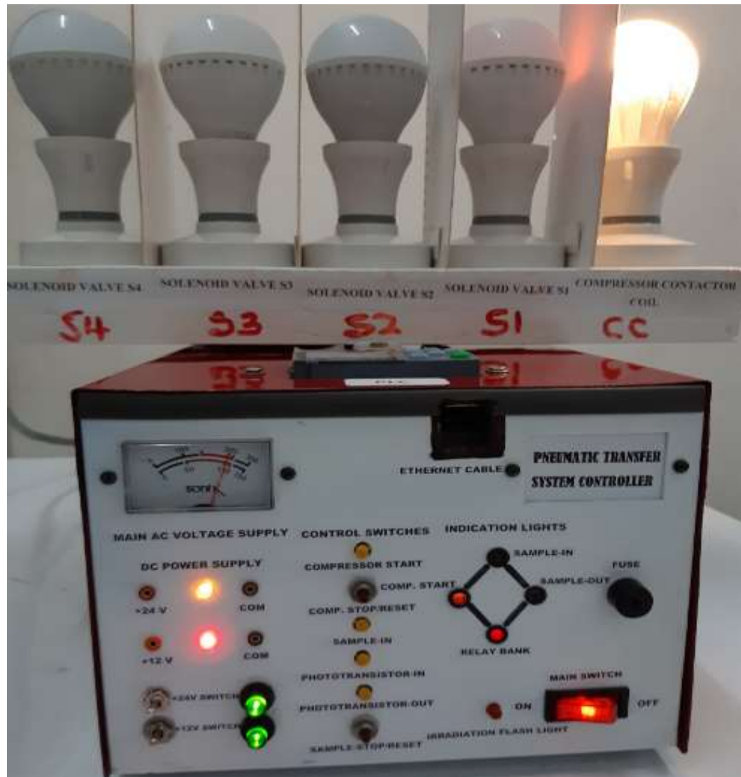
Figure 72: Contactor coil energized, compressor starts.
