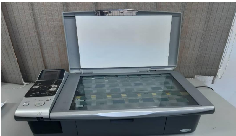
Figure 14: Epson Stylus Scanner with Strips of Irradiated Gafchromic EBT3
