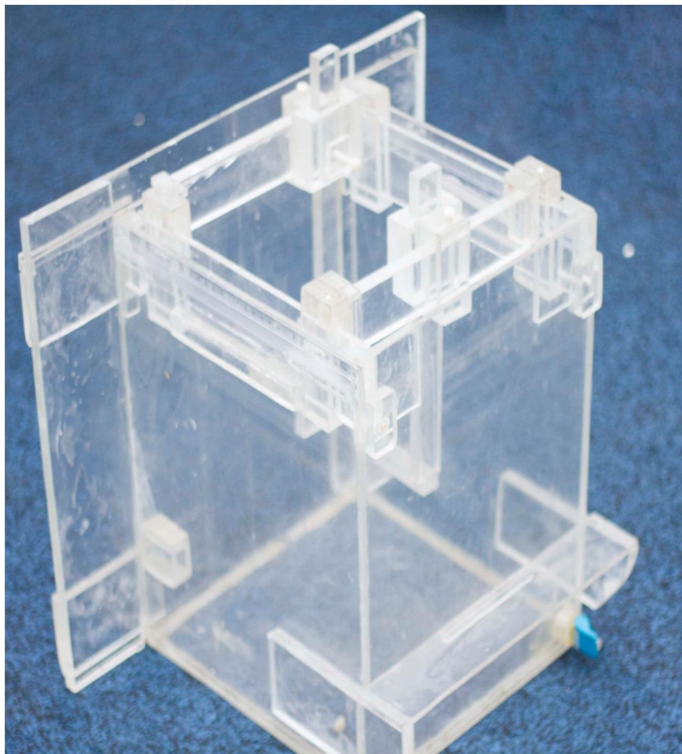
Figure 17: 3D View of the Constructed Water Phantom
