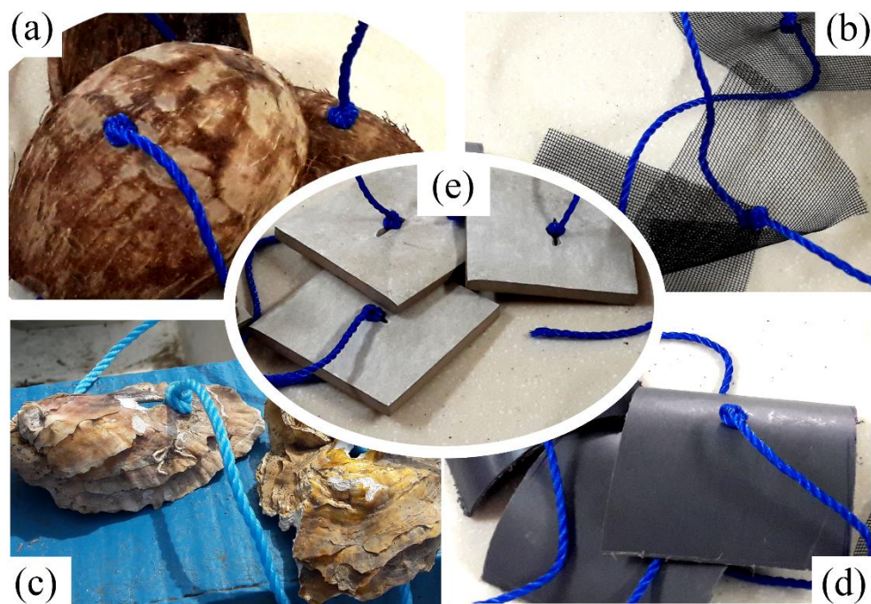
Figure 3.4: Oyster spat collector materials tested for effectiveness (a) coconut shell, (b) fine mesh nylon net (mosquito net), (c) oyster shell (recycled), (d) PVC slats and (e) ceramic tiles.
