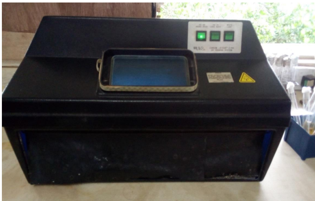
Plate 2: A Typical Setup for the Batch Reaction Under UV Light Irradiation High Performance Liquid Chromatography (HPLC) Analysis of the Parent Ethylparaben
