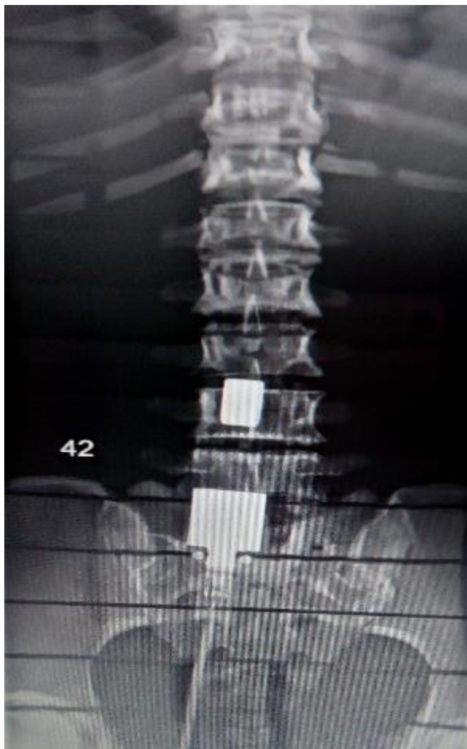
Figure 4.23: Image Showing Lumbar Spine AP Acquired from Rando Female Anthropomorphic Phantom at 70 kVp, 22 mAs, ESD = 1.94 mGy, EI = 679.
