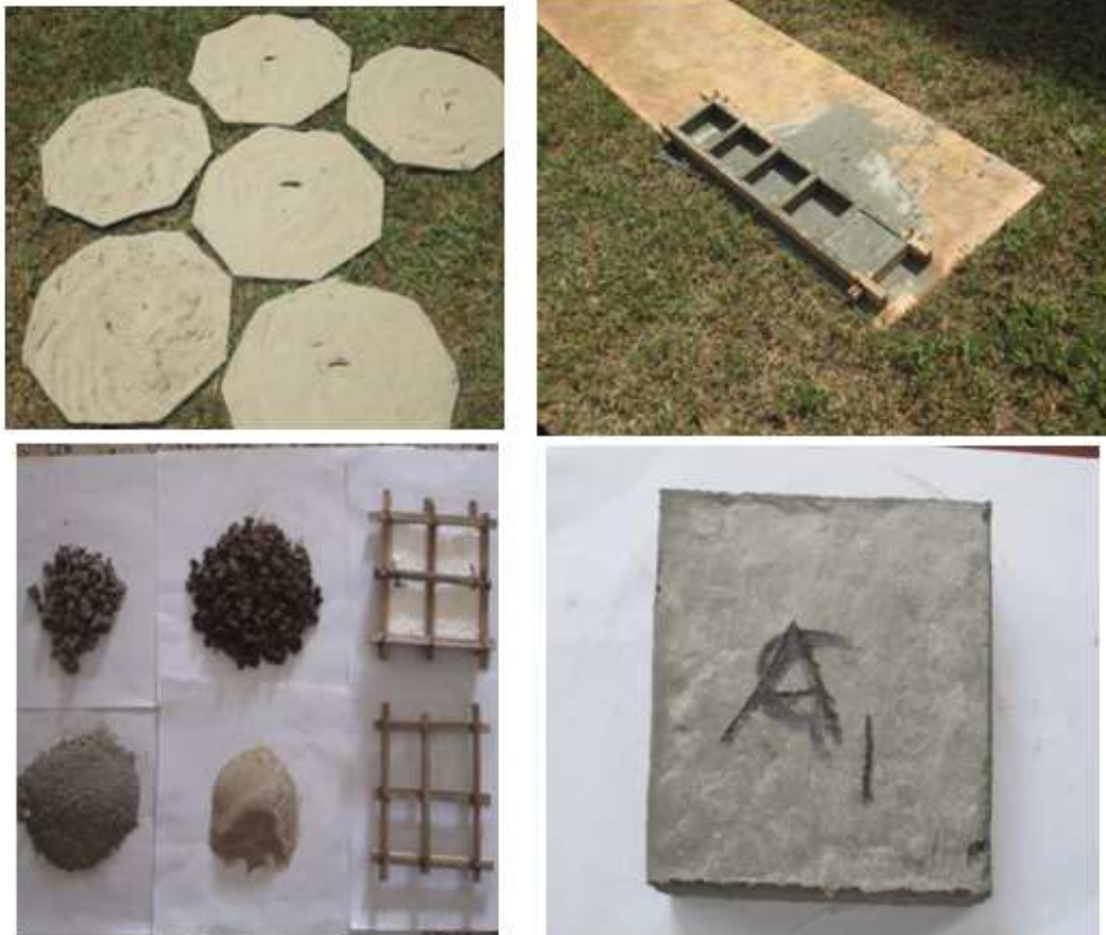
Pictures showing samples of the raw materials used in the production of the slabs. This follows in the order, sand preparation, slab- mold, stone and bamboo mesh and concrete slab.
