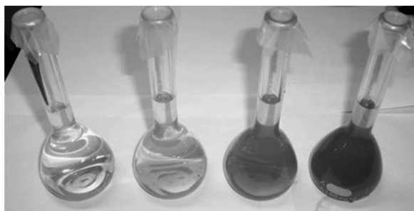
FIG. 7. Color variation of solutions of different turbidity following 20 \times dilution (from left to right 50, 100, 250, and 500 mg/L initial selenium concentration).
