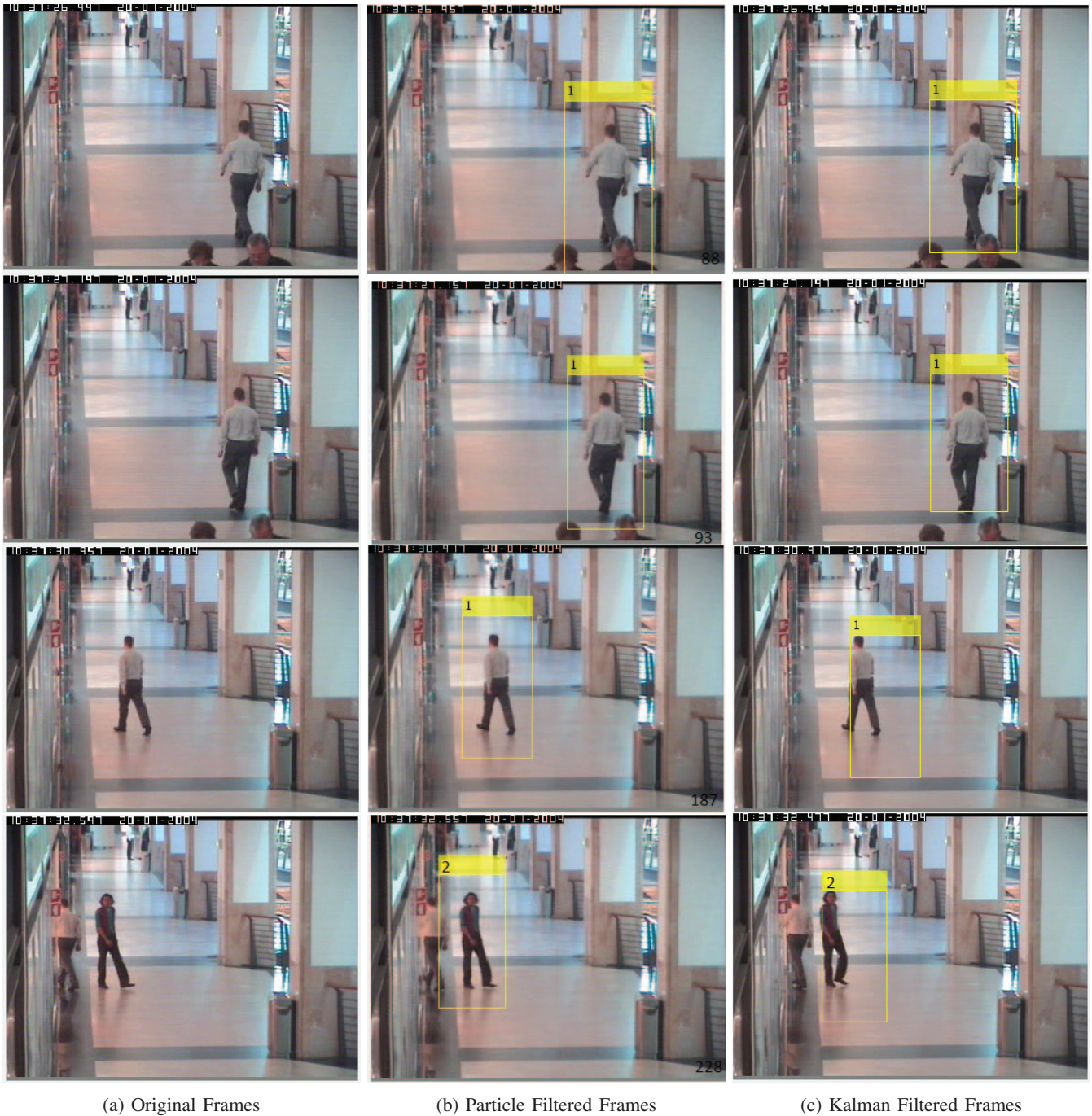
Fig. 1: The figures show people tracking at work on some selected frames. (a) The first column shows the original frames (b) The second column shows Particle filtered frames (c) The Kalman filtered frames. Analysis of the bounding boxes placement during tracking shows the Particle filtered tracking is better.
