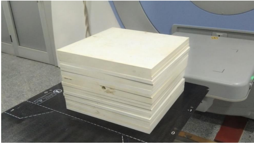
Figure 1: Pack of 30 \times 30 cm 2 PMMA phantom slabs used in this study.
