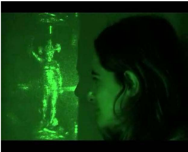
Fig. 23 A spectator observing the acquired holograms SLM optical reconstructions, projected on a screen. The size of the image reconstructed at visible wavelength was about 30 cm, comparable to the original object size
