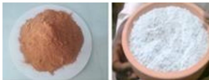
Fig. 1 Raw materials (left): bauxite from Awaso bauxite mine, (middle): kaolin from Awaso bauxite mine and (right): kaolin from Anfoega (all in Ghana) used for zeolite synthesis
