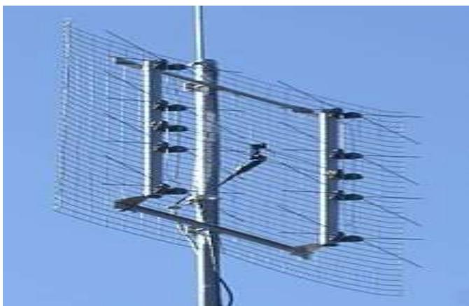
*Figure 10: A photograph of a Reflective array antenna*
