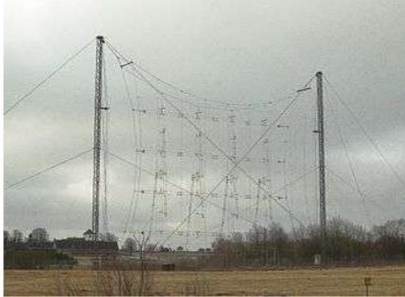
*Figure 12: A photograph of a Curtain array antenna*
