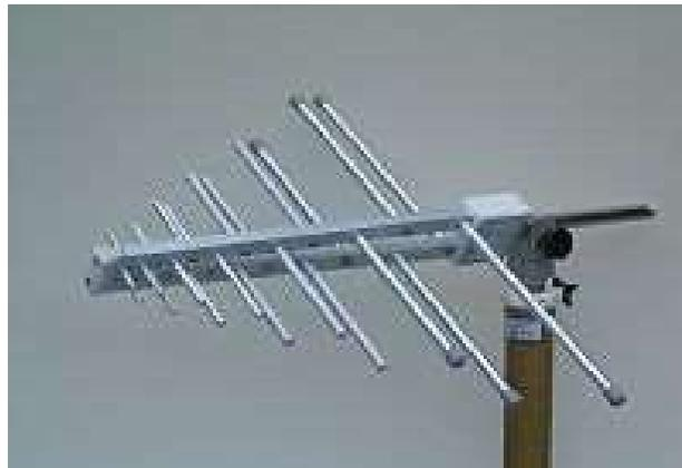
*Figure 9: A photograph of a Log-periodic antenna*
