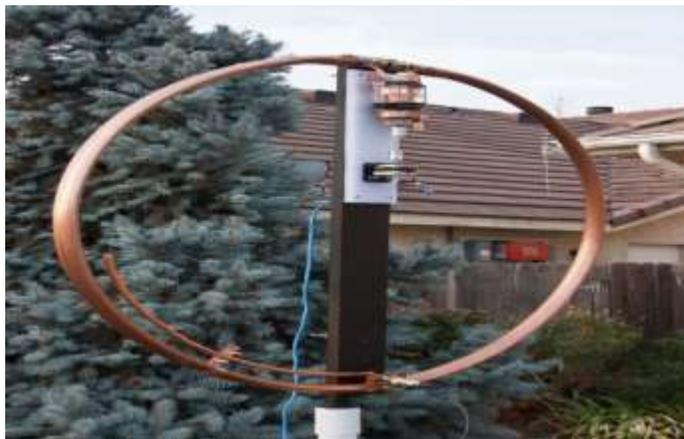
*Figure 15: A photograph of a large loop antenna*
