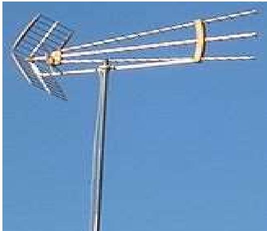
*Figure 4: A photograph of a corner reflector antenna*
