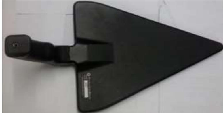
*Figure 30: A photograph of log-periodic antenna model TS-6021*
