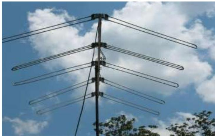
*Figure 19: A photograph of a Traveling wave antenna*
