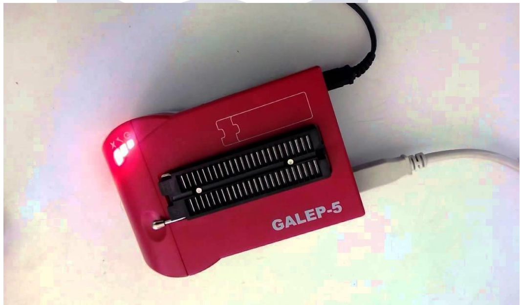
Plate 6: Galep-5 Programmer used to write the program unto the microcontroller and the IC
