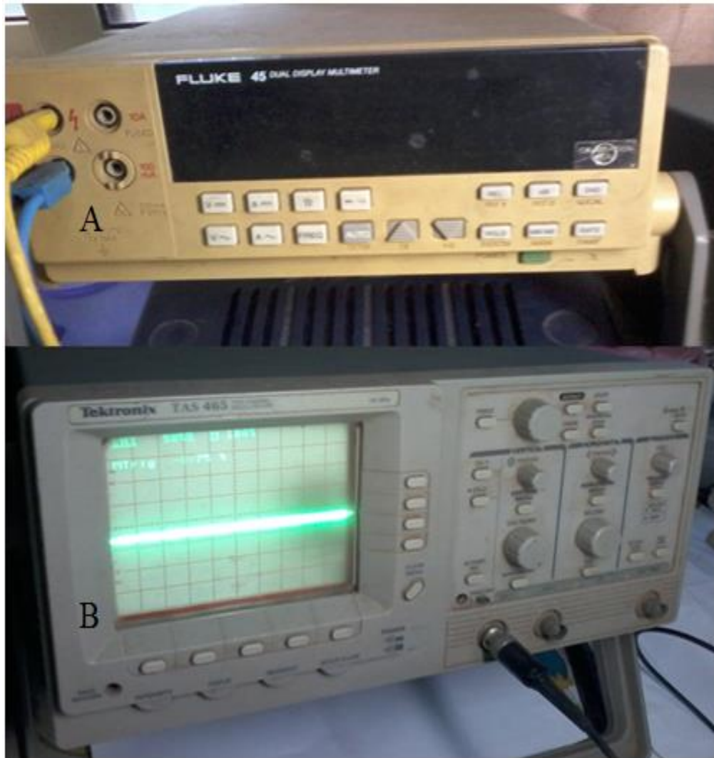
Plate 1: Measuring Instruments used for measuring voltages and waveforms during the Data acquisition stage of this work; A) Digital Multimeter; B) Tektronix Oscilloscope.
