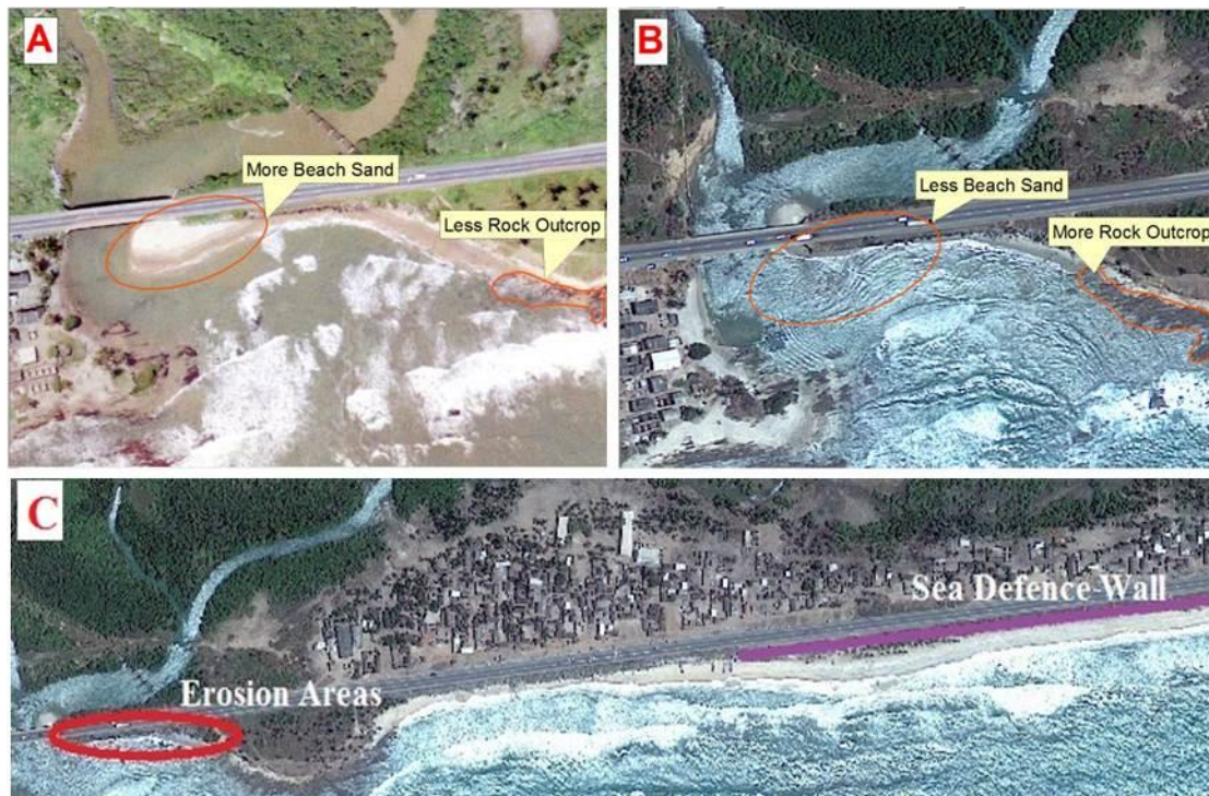
374 Figure 11: Erosion of sandy beach at the Elmina Highway Bridge. (A) shows more sand at 375 the Elmina Bridge in 2005 which was eroded by 2011, (B) with further exposure of 376 underlying rocks, (C) shows section of the 1.5 km rock revetment sea defence near the 377 Elmina Highway Bridge.
