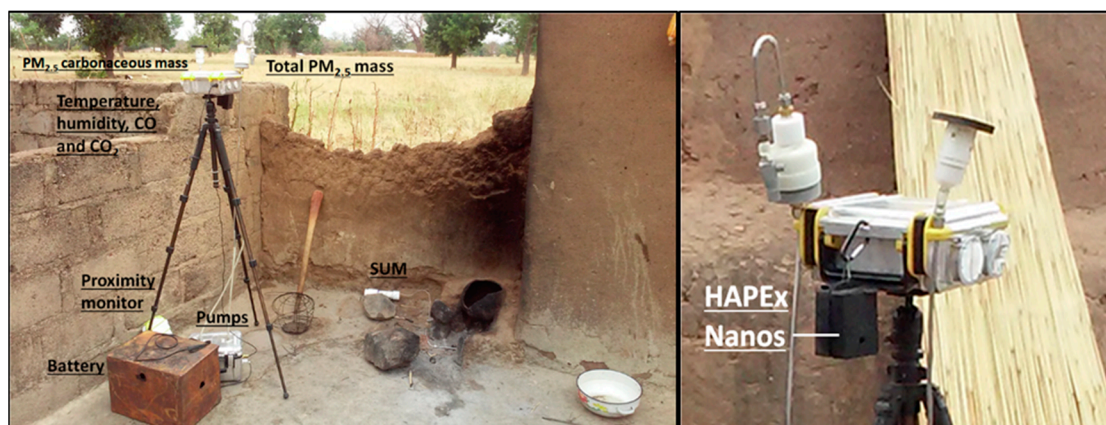
Figure 1. Microenvironment sampling apparatus deployed at a typical rural kitchen in the Kassena-Nankana (KN) district. Additional monitoring instrumentation is shown including a stove use monitor (SUM) and participant proximity monitor.
