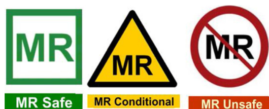
Fig. 6. Symbols for device labeling terms (MR safe, conditional, and unsafe).
